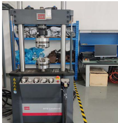
Figure 3. MTS Landmark Electro-hydraulic servo dynamic test system 图 3. MTS Landmark 电液伺服动态测试系统
