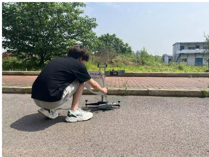
**Figure 8.** Swing instrument determines the road surface friction coefficient
