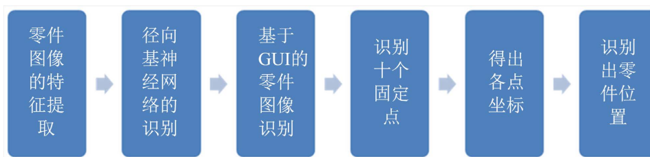
Figure 11. Coordinate method recognition time step diagram 图 11. 坐标法识别时间步骤图
