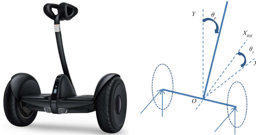
Figure 1. Two wheeled-self balancing robot coordinate system 图 1. 两轮自平衡机器人坐标系
