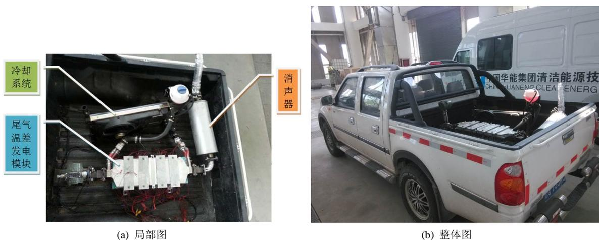
Figure 3. ATEH is shown for the automobile test system in the laboratory pictures at below: (a) zoom-in; (b) overview
