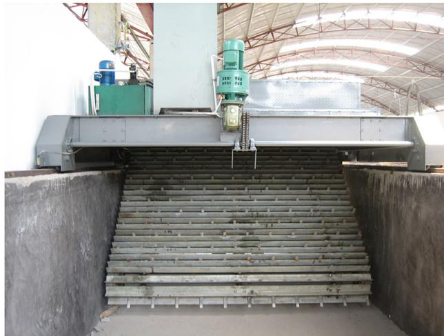
Figure 2. Trough dumping composting system
