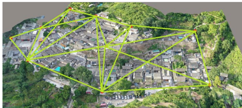
Figure 3. Contemporary landscape and 3D mapping control network of Cuandixia Village 图 3. 爨底下村当代景观及三维测绘控制网
