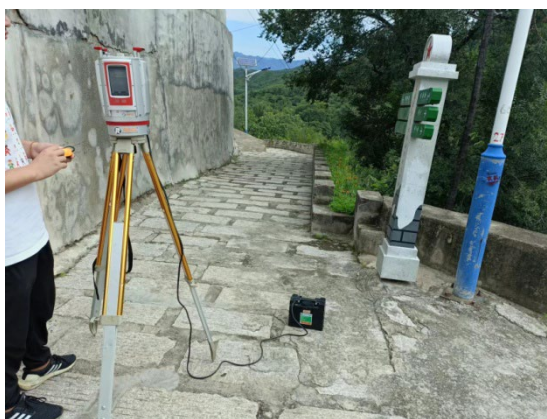
Figure 6. 3D laser scanning
