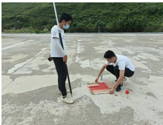
Figure 5. UAV image control point layout
