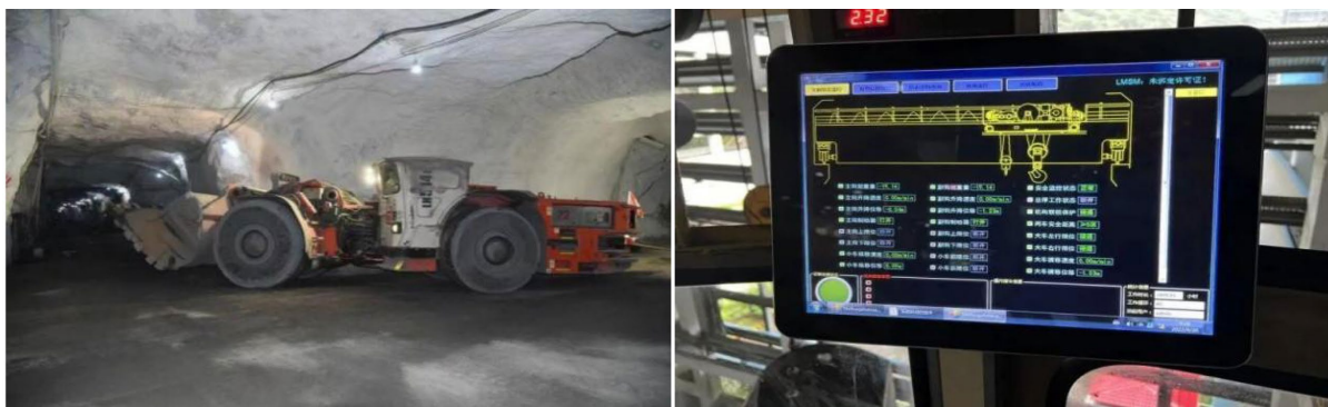
Figure 5. Unmanned electric shovel in underground mine
