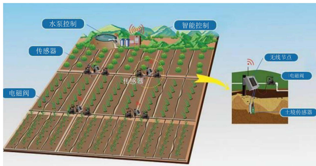
Figure 2. On-site deployment diagram of intelligent irrigation equipment 图 2. 智能灌溉设备现场部署图
