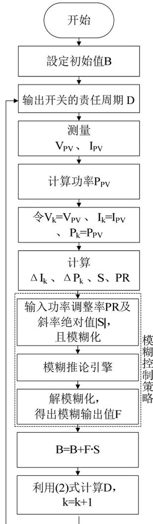
Figure 8 Flowchart of the fuzzy-based tracking algorithm
