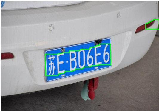
Figure 6. Contour search and drawing effect drawing 图 6. 轮廓查找与绘制效果图
