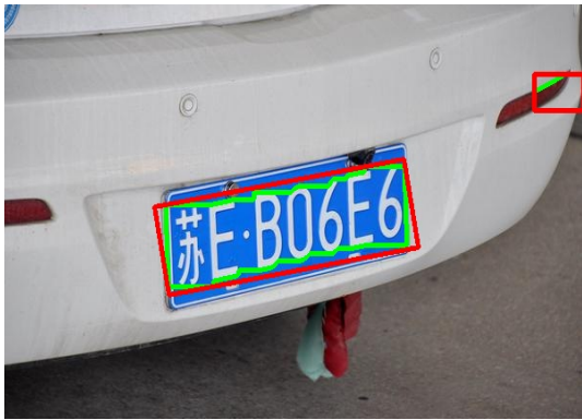
Figure 7. Minimum circumscribed rectangle detection effect drawing 图 7. 最小外接矩形检测效果图
