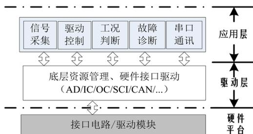
Figure 2. Software structure design diagram
