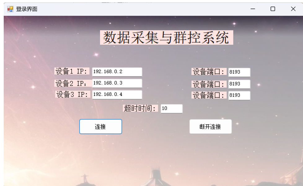
Figure 5. Connection interface between control and data acquisition system and CNC machine tool 图 5. 控制与数采系统与数控机床的连接界面
