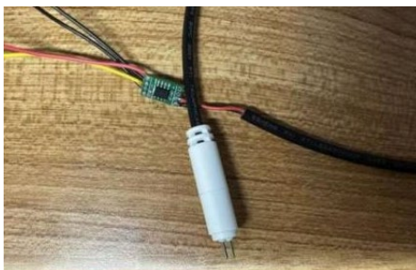
Figure 5. Conductivity detection module 图 5. 电导率检测模块
