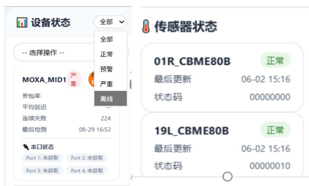
Figure 8. Detailed interface for equipment and sensor status 图 8. 设备与传感器状态详细界面
