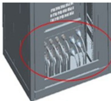
Figure 3. Internal transfer panel diagram of prefabricated cabin 图 3. 预制舱内部转接面板示意图
