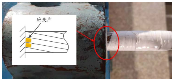
Figure 3. Strain sensors on the conductor at the end 图 3. 应变片在导线端部的粘贴方式
