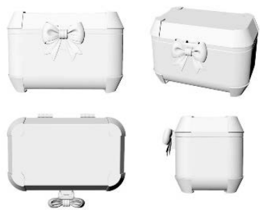
Figure 2. Waterproof side box with double-layer sealed structure design 图 2. Q5 防水边箱双层密封结构设计
