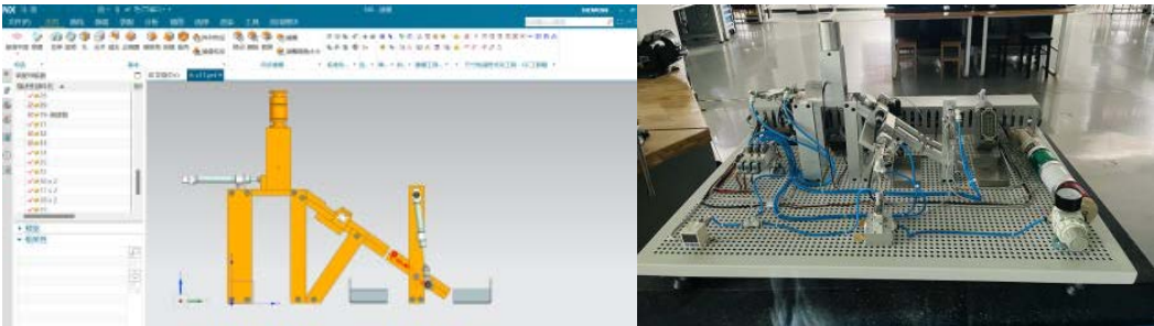
Figure 3. Three dimensional model of the mechanism and solid stator sliding compartment sorting system 图 3. 机构三维模型与实体定子滑仓整理系统
