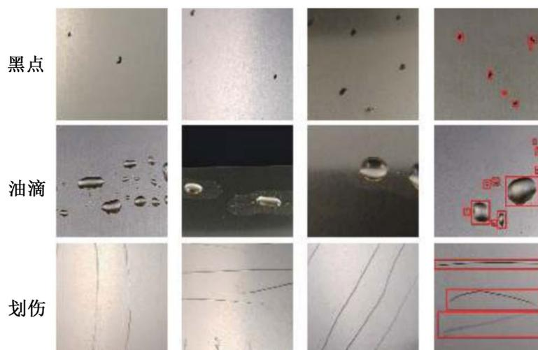
**Figure 3.** Examples of three types of defect images in KMUST-DET data set
