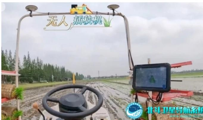
**Figure 3.** Beidou Satellite Navigation System terminal helps unmanned agricultural machines to carry out precise seeding
