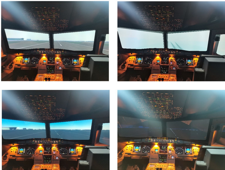
Figure 4. Exterior display of flight simulator under different visibility scenarios 图 4. 不同能见度情景下飞行模拟器外景展示
