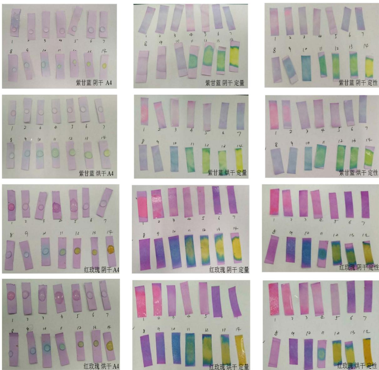
**Figure 3.** Color of pH 1~14 solution with self-made acid base test paper
