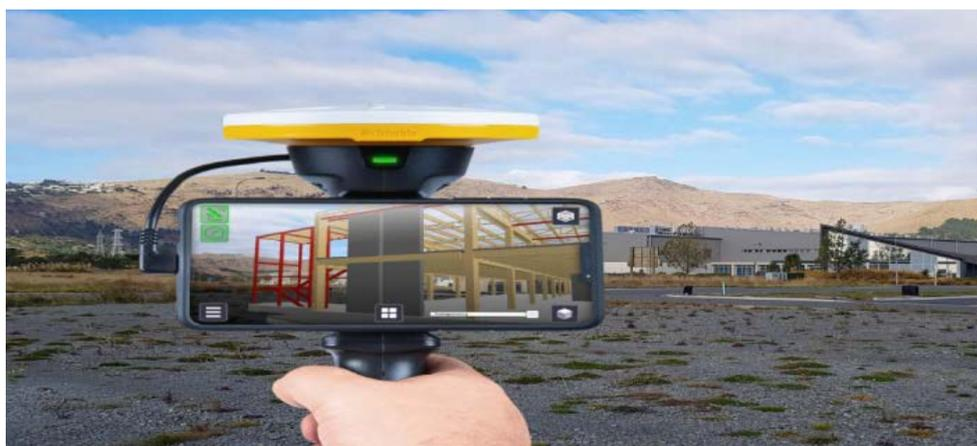
Figure 4. The MR technology superimposes the completed building renderings onto the actual construction site
