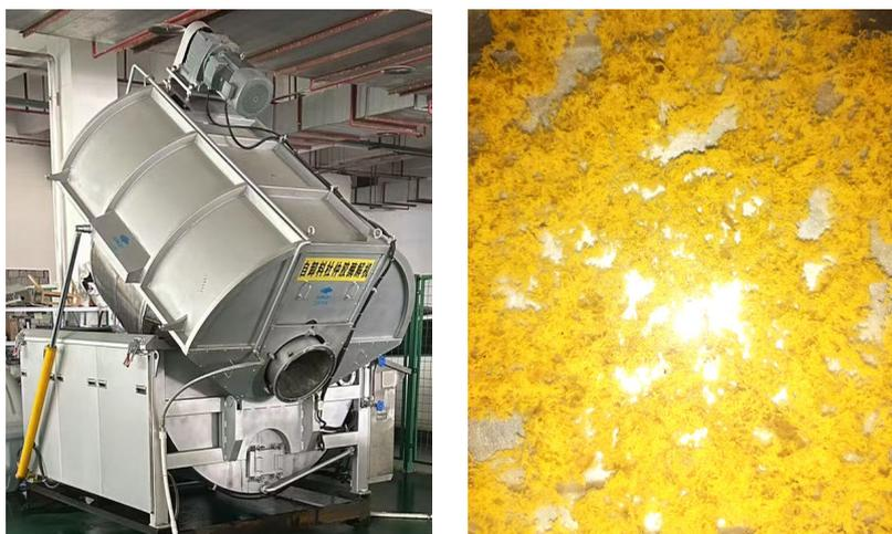
Figure 7. Self-discharging *Eucommia* enzyme hydrolysis purification machine and the extracted leaf gum
