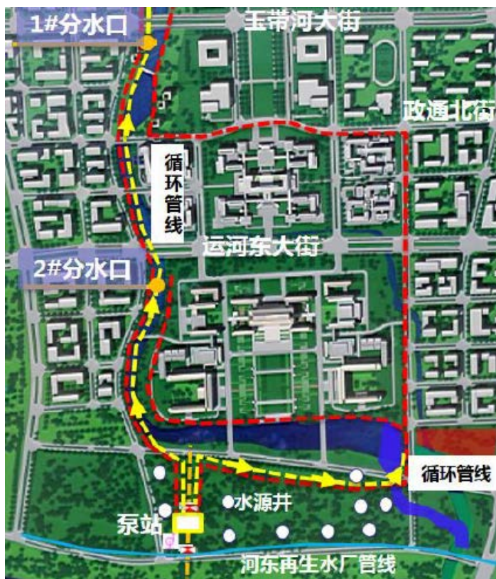
Figure 2. Schematic diagram of the location of the circulation pipeline, distribution outlet, and water source well 图 2. 循环管线、分水口及水源井位置示意图
