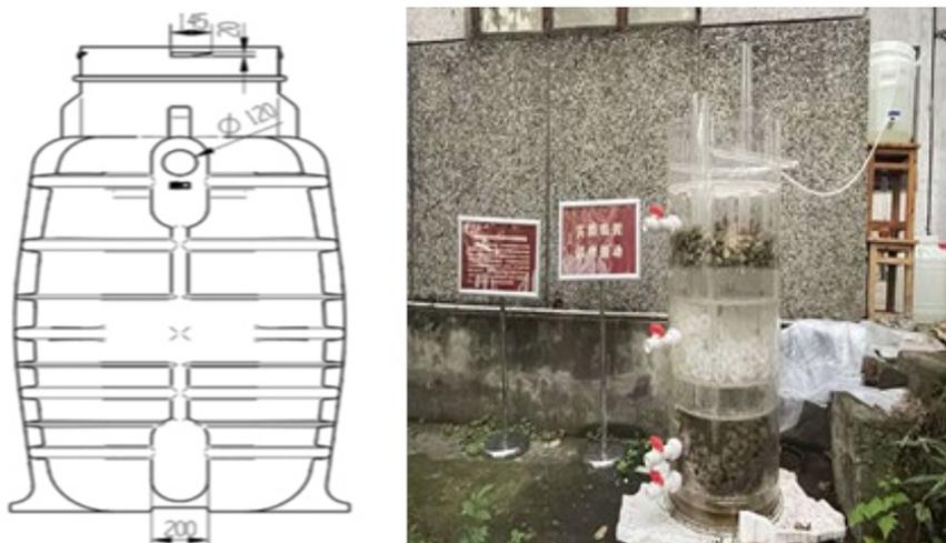
Figure 1. Schematic and actual view of the non-powered wastewater treatment system
